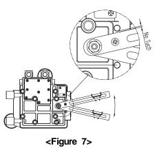
(9) After the proper installation, tighten all of the bolts on the bracket, the feedback lever, and the connection bar.
