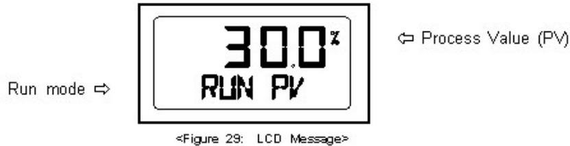
"RUN" indicates that YT-2300 adjusts valve stroke with receiving signals (4~20mA) and "PV" indicates the process value. In RUN mode, the valve stroke continuously changes according to the input signal. There are six types of display message in RUN mode. <Figure 30>
